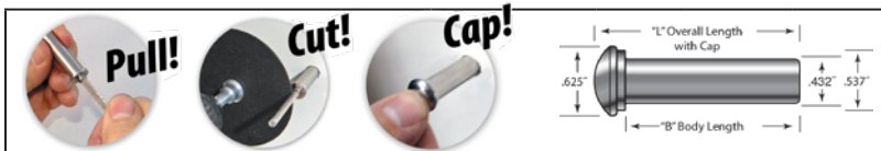
Hidden Pull Locking Fitting - for 1/8" or 3/16" cable
