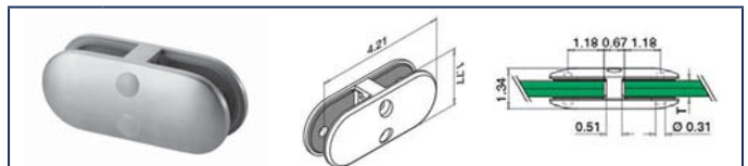
Model 28S - Glass Clamp Straight (glass to glass) 1.35" thick x 1.77" high x 4.21" long.
